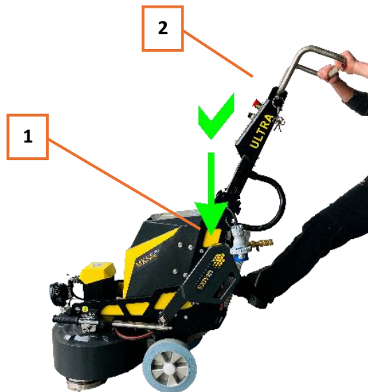
Fig. 33 Machine with vertical guide and control console
