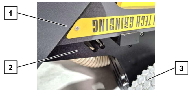
Fig. 7 Fixing point for the locking bolt - tilting position
